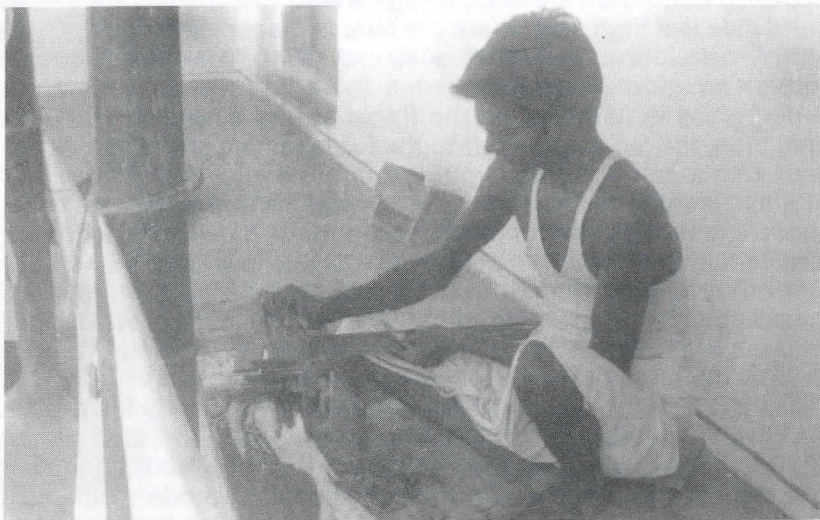
Plate 7: PAPANAIIDUPET Cutting the tubes into bead sizes.
