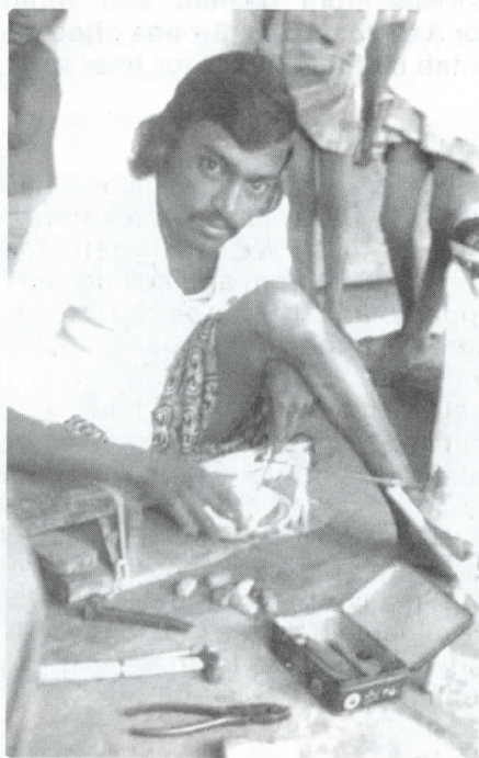
Plate 4: CAMBAY Himmat Patel of Nagara demonstrates the boring of stone beads.
