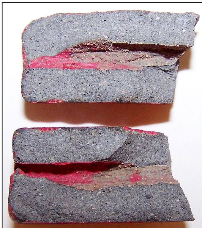
**Figure 4. Fracture surface of a painted cement bead.**
