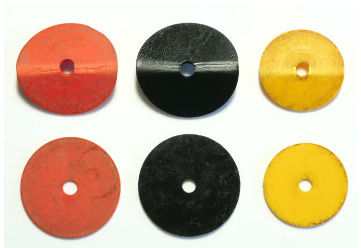
Figure 9. PVC disk beads. The top row shows damage after flexing a few times. Bead diameter 12 mm (red and black); 10 mm (yellow).
