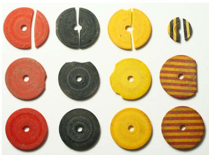
Figure 4. Celluloid disk beads. Fractured beads and beads with chipped edges are shown to illustrate the failure mode and typical age-related damage. Bead diameter 11.2 – 11.5 mm.
