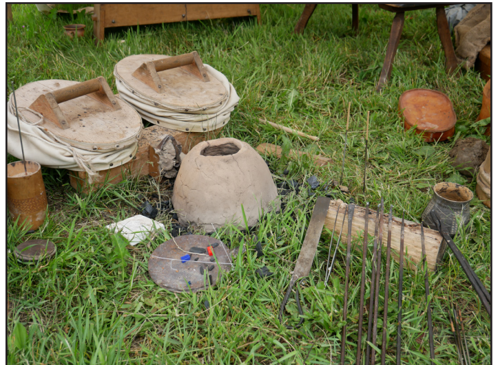
Figure 2. Viking-type furnace with bellows. Photo by author.
