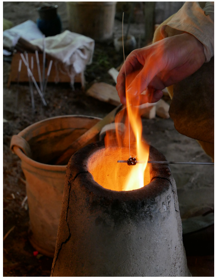
Figure 4. A wound bead is decorated above a volcano-type furnace with dot decorations using a thin strand of glass. Photo by author.
