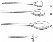
is required for thermometers, the first ball is flattened by an iron or wood battledore, on the marver, prior to the subsequent gatherings; this ensures a flat bore, although the exterior of the tube is round. The ball is then elongated by
